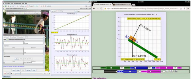
Figure 4. Practice 2: Use Models such as existing Easy Java Simulation models for example the sliding frictional model on the right is available https://dl.dropboxusercontent.com/u/44365627/lookangEJSworkspace/export/ejs_model_friction/friction Simulation.html
